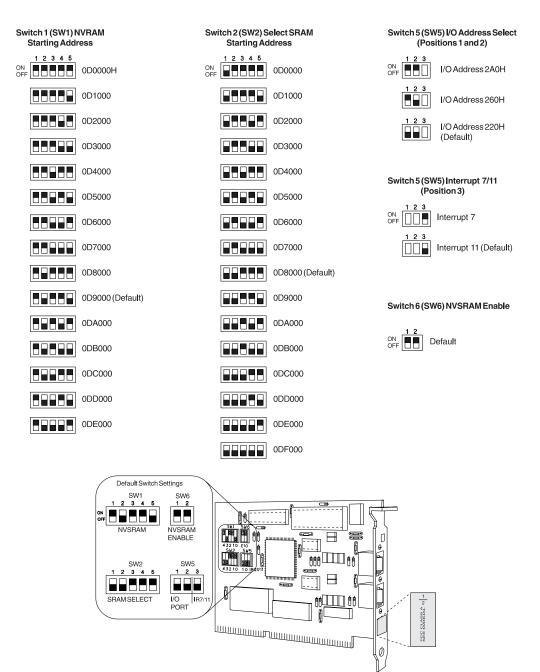
Figure 1. Point of Sale Attachment Adapter Switches
