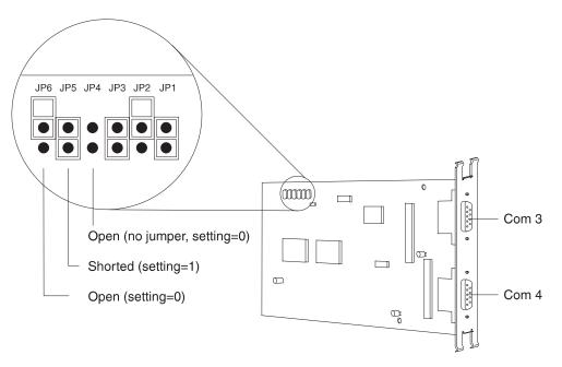
Figure 3. 4695 RS232 Expansion Adapter Jumpers
