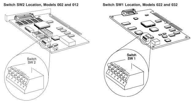
4. See Table 1 and Table 2 on page 8 to set the switches on **SW1** or **SW2** to match the configuration to the memory map.
