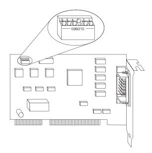
Figure 2. Flat Panel Display Adapter Switch Settings
