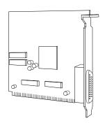
Figure 5. Parallel Port Adapter
