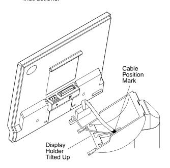
Figure 1-2. Display Holder Tilted Up
