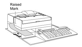
Figure 2-13. Inserting a Document at the Side of Model 2 Printer
