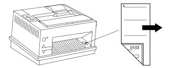
Figure 2-21. Model 4R Printer With Check Orientation Label
