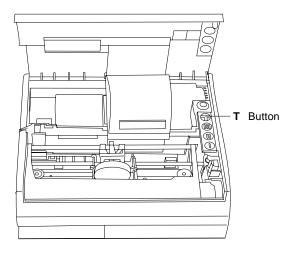
Figure 2-14. Test Button on Model 2 Printer
