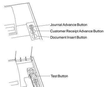
Figure 2-11. Buttons on a Model 2 Printer
