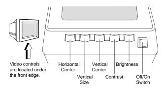
Figure 2-3. Controls on 9-Inch Color Display
