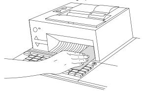
Figure 2-22. Inserting a Check in the MICR Printer
