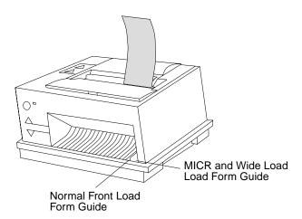
Figure 2-18. Inserting a Document at the Top of Model 4 Printer
