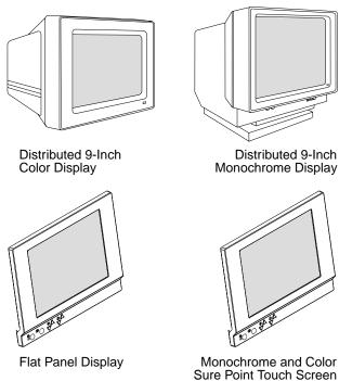
The Sure Point Touch Screens are 9.5 inch liquid crystal displays with a touch screen panel. They can be setup in an integrated arrangement or they can be placed by themselves in a distributed arrangement.
