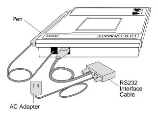
Figure 1-6. Signature Capture Device RS232 Interface Model
