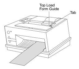
Figure 2-17. Inserting a Document at the Front of Model 4 Printer
