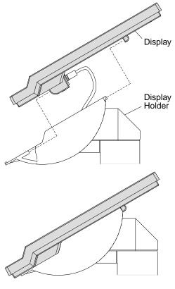
Figure 1-3. Installing the Display Unit
