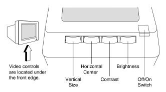
Figure 2-2. Controls on 9-Inch Monochrome Display
