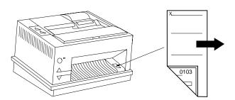
Figure 2-23. Check Orientation Label on Printer
