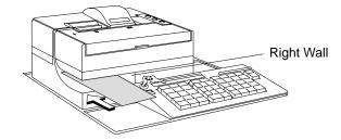
Figure 2-12. Inserting a Document at the Front of Model 2 Printer
