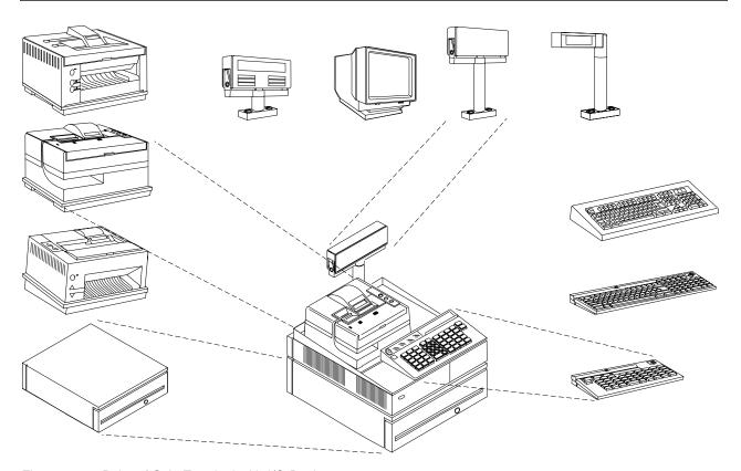
Figure 1-1. Point-of-Sale Terminal with I/O Devices
