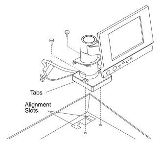
Figure 1-5. Integration Kit with Display Attached
