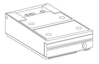
The flip-top cash drawer, is smaller in size. It can be used in distributed arrangements where space may be limited. Its top cover hinges up. It, too, can have an optional keylock to permit the top cover to open under application program control or by means of a key.
