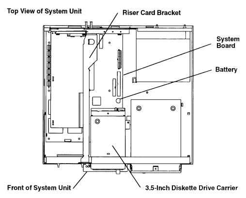
3. Push the edge of the battery toward the center of the system board until the edge clears the sides of the battery container, and then lift the edge of the battery upward; remove the battery.
