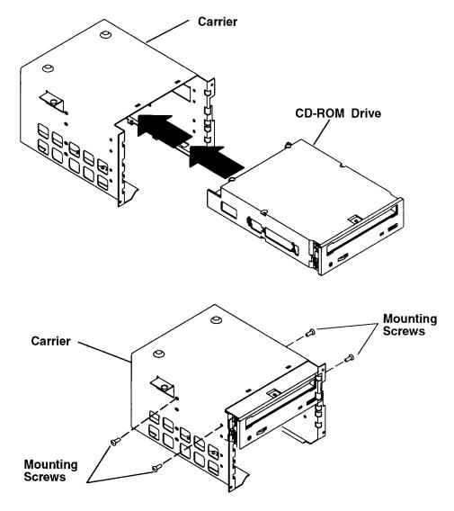
8. Place the disk drive in the bottom position of the carrier, and then install the four mounting screws through the bottom of the carrier and into the disk drive.
