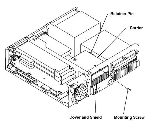
6. Connect one end of the signal cable to the connector on the rear of the 3.5-inch diskette
