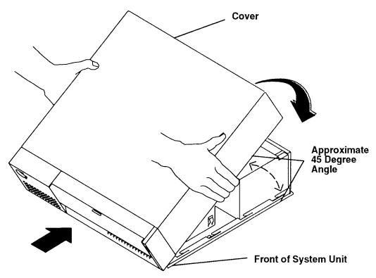
4. Slide the cover toward the rear of the system unit until the cover stops and the cover screw holes are against the chassis screw holes.
