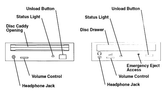
When the CD-ROM is set to On, the status light indicates one of several conditions. The following are status light states and the respective conditions of the CD-ROM drive:
