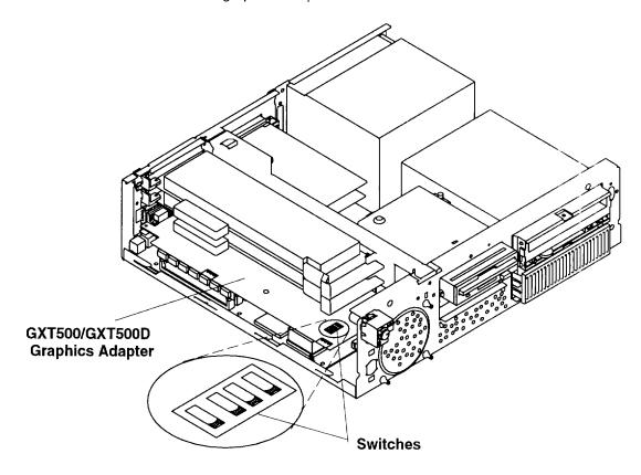
3. The following table describes how to set the switches on the POWER GXT500/POWER GXT500D graphics adapter for use with the various displays. Find your display type in the table and look up the correct switch settings in the Adapter Display Switch column.
