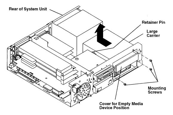
7. Place the CD-ROM or tape drive in the desired (top or bottom) position of the carrier, and then install the four mounting screws through the carrier and into the media device.
