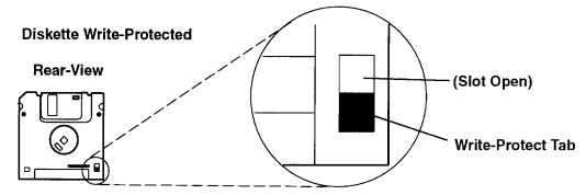
• To allow writing onto a diskette, slide the write-protect tab to cover the protect slot.
