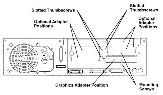
4. Slide the cover for the empty adapter position toward the side of the system unit, and then remove it. Retain the cover for possible future use.
