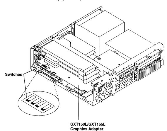
3. The following table describes how to set the switches on the POWER GXT150L/POWER GXT155L graphics adapter for use with the various displays. Find your display type in the table and look up the correct switch settings in the Display Switch column
