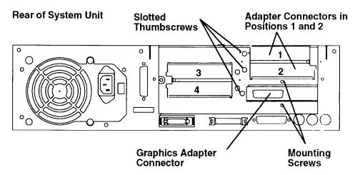
d. Grasp the plastic handles, pull the adapter out of the slot on the riser card, and then remove the adapter out of the system unit.
