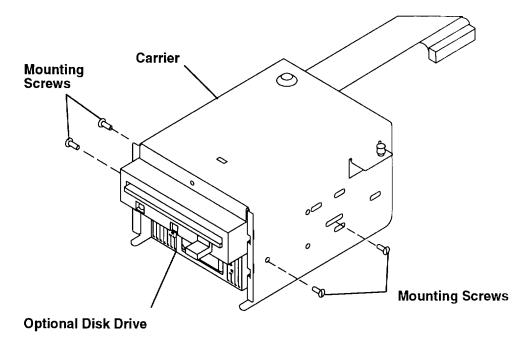
9. Place the front of the 3.5-inch diskette drive through the opening in the chassis, and then place the mounting tabs of the carrier through the slots in the front of the chassis.
