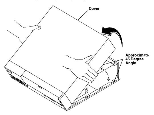
13. While keeping the cover tilted at approximately a 45 degree angle, slide the cover forward until the cover clears the front of the system unit, and then lift the cover away from the system unit.
