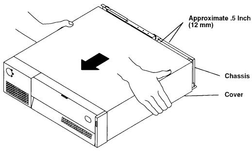
12. Grasp both sides of the cover, and then rotate the rear of the cover upward until the cover is tilted at approximately a 45 degree angle.
