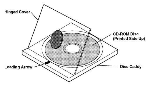
With the loading arrow toward the drive and the printed side of the disc up, insert the caddy in the disc caddy opening. Push gently on the caddy. The drive automatically pulls the caddy into the drive and prepares the disc for reading.
