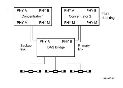
Figure B-8: DAS Bridge Installed for Dual Homing
