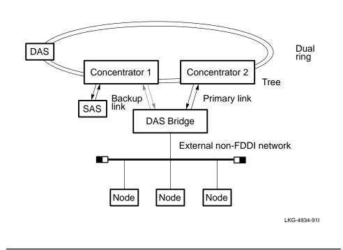
Figure 1–18: Dual Homing Topology Using Concentrators and a DAS Bridge
