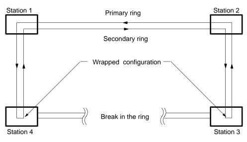
Figure 1–14: Dual Ring—Isolating a Link Failure
