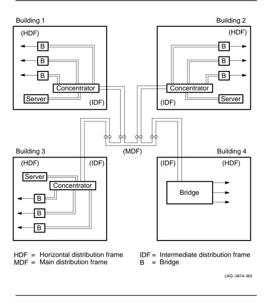
Figure B–6: Dual Ring of Concentrators and Bridges Installed in a Campus
