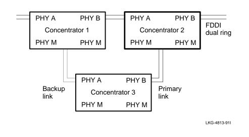
Figure B-7: Concentrators Installed for Dual Homing
