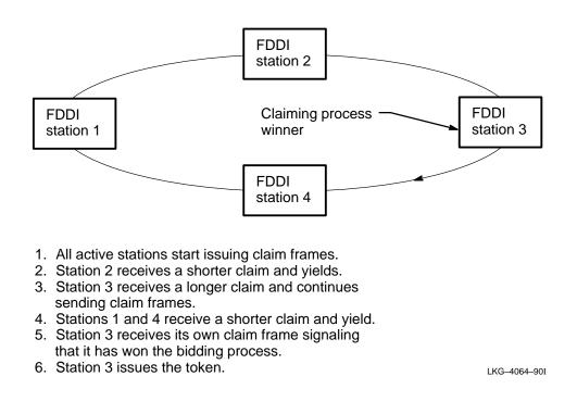
The claiming process determines which station will initialize the ring. The process begins when one or more MACs enter the claim state. In this state, the MAC continually transmits claim frames. The claim frame contains the originator's address and the station's bid (called T\_Bid) for TTRT.
