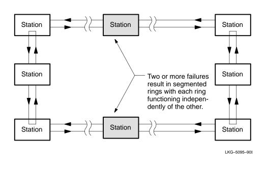
Figure 1–20: Dual Ring Failure of an FDDI Topology
