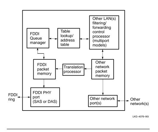
Figure 4–2: FDDI Bridge Functional Diagram
