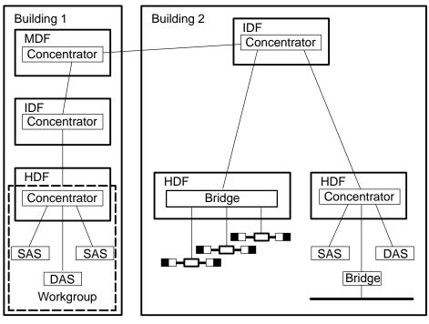
HDF = Horizontal distribution frame IDF = Intermediate distribution frame MDF = Main distribution frame SAS = Single attachment station DAS = Dual attachment station
