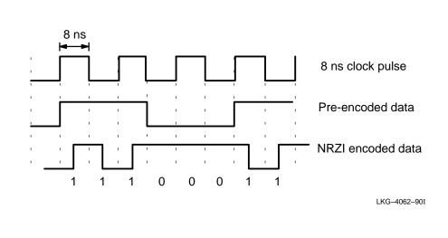
Figure 2–5: NRZI Encoding Process
