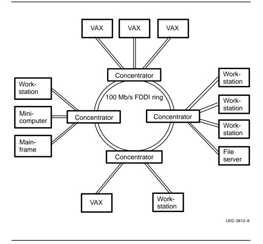
Figure B-5: Dual Ring of Concentrators Installed in a Building
