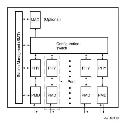
Figure 3–3: Concentrator Architecture
