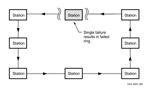
Figure 1–19: Single Ring Failure of a non-FDDI Topology
