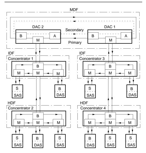
DACs1 and 2 are connected through PHY ports A and B to the dual ring. Concentrators attach to the ring through PHY ports M and B. DASs connect to the ring through PHY port B. DAS PHY port A is not used in this topology. Arrows indicate direction of token flow.
