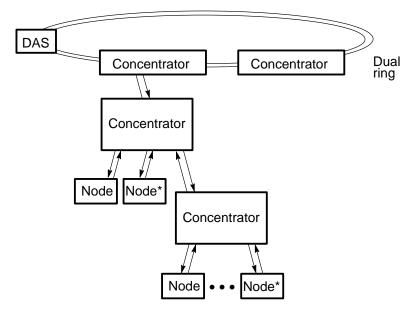
\* Multiple station failures in a dual ring of trees result in no loss of access to the ring. Failing stations are simply removed from the ring.
