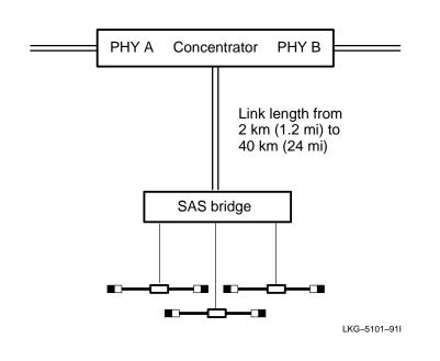
Figure B–9: Connecting to the Dual Ring Through a Single-Mode Link
